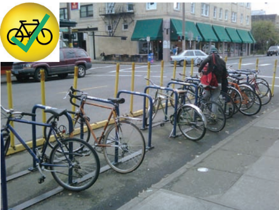
Fig. 19: Replacing one automobile parking space with standard U Racks can yield as many as twelve bicycle parking spaces.
