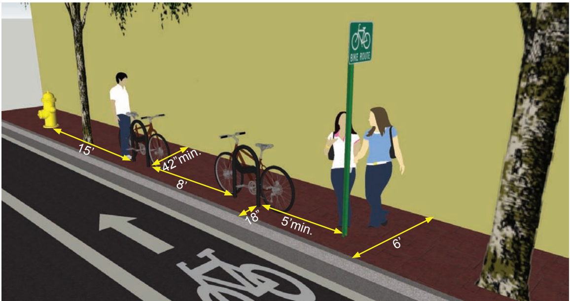
Fig.38: The above dimensions provide specific siting guidelines for bicycle parking within a constrained streetscape.
