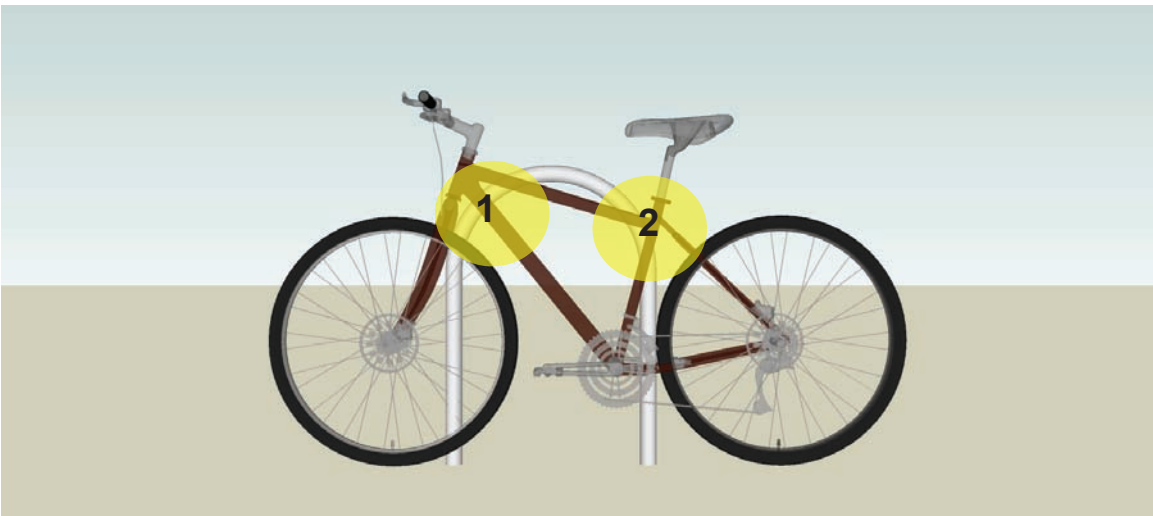
Fig. 8: An acceptable bicycle rack allows the frame to support and secure the bicycle with a standard U-lock or cable lock in at least two places.
