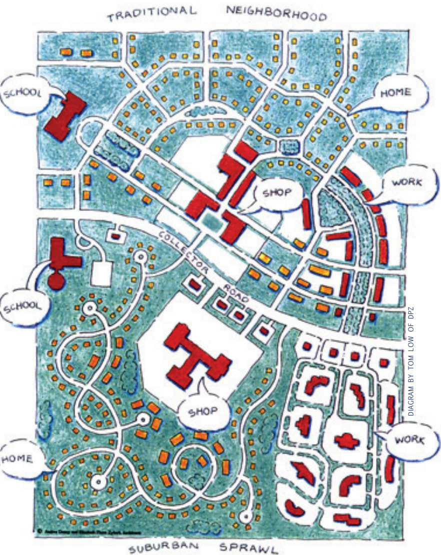
Diagram of some of the plan differences between form based codes (top), and conventional use based codes (bottom). Both contain the same uses, but the form based plan is interconnected, mixed use, and places buildings to create walkable streets and squares.
