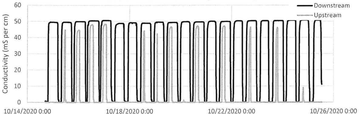
FIGURE 2 – TIDAL DATA COLLECTION IN CASTNER BROOK AT CHURCH STREET RECORDED CONDUCTIVITY (mS PER CM)
