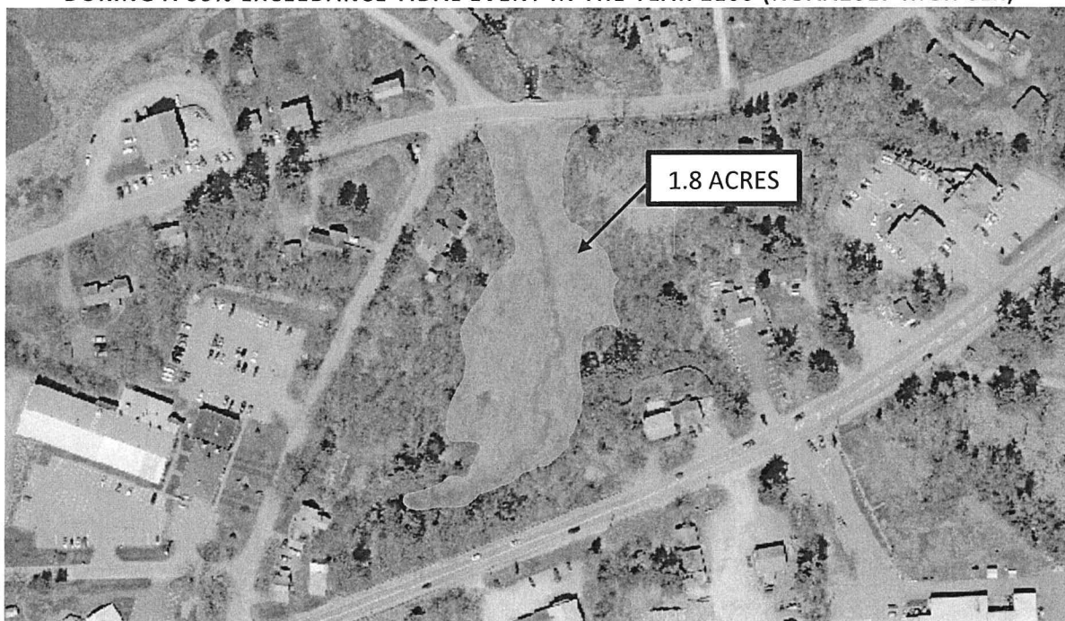
FIGURE 5 – AREA OF POTENTIAL TIDAL INUNDATION UPSTREAM OF CHURCH STREET DURING A 99% EXCEEDANCE TIDAL EVENT IN THE YEAR 2100 (NOAA2017 HIGH SLR)
