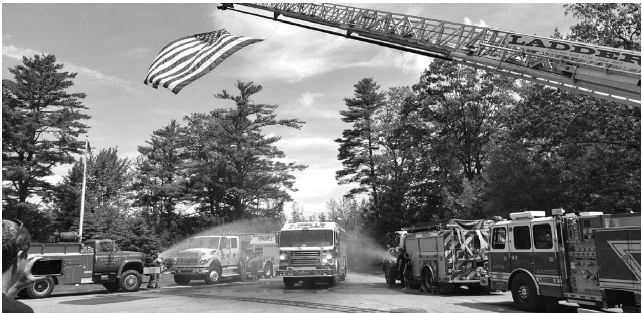
Engine 2 (2018) at the wet-down ceremony. It is equipped with a 1,500 gallon per minute pump, 1,000 gallons of water with a custom 5 man cab. The onboard generator will power Jaws of Life and the truck will carry all of the rescue equipment for the Engine Company as well as a full compliment of firefighting tools.
